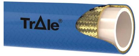
**Composition:** •Inner tube: polyamide. •Reinforcement: one braid of steel wire. •Cover: blue polyurethane.
